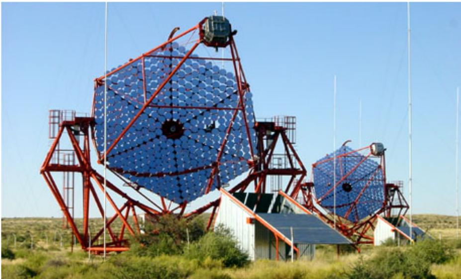
*Picture of 2 H.E.S.S. telescopes*
