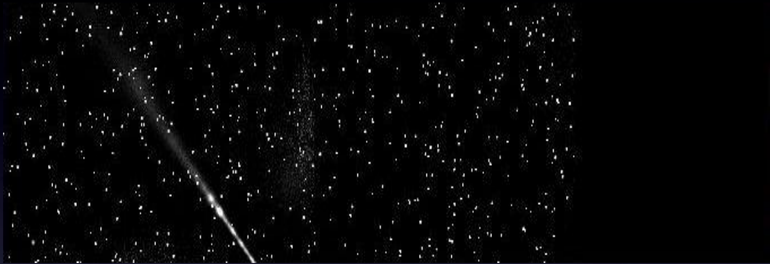
X-ray image using a ^{55}\text{Fe} source CCD Overscan
