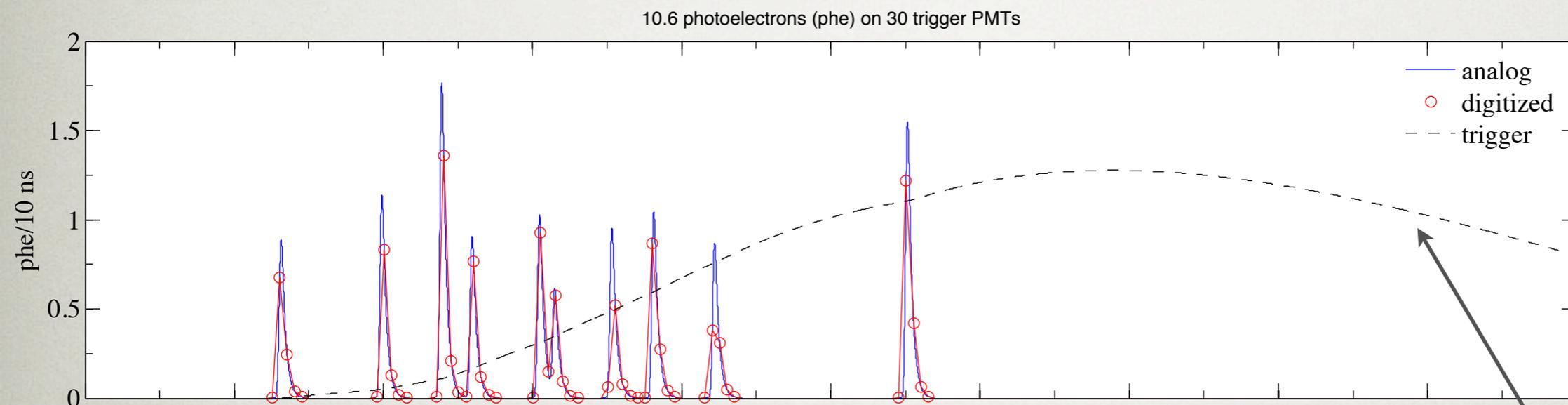
Shaped analog signal for trigger hardware
