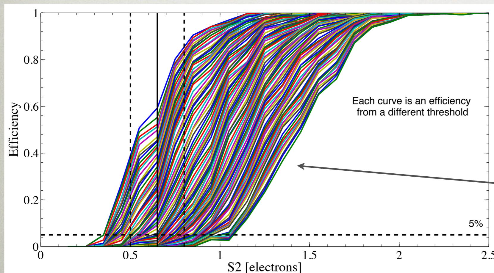
Adjusting the trigger set point gives different detection efficiency curves. Can quantify the curve by the point there it crosses 5%, or the "turn-on".
